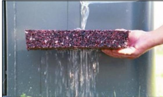
*Pervious pavement is highly permeable while maintaining structural strength..*
